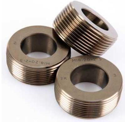
Our stocked thread rolls are manufactured from M2 High speed steel hardened to HRC 62-64. We also stock some thread rolls in M42. These are only for UNJF threads that are normally used on tough aircraft materials.
