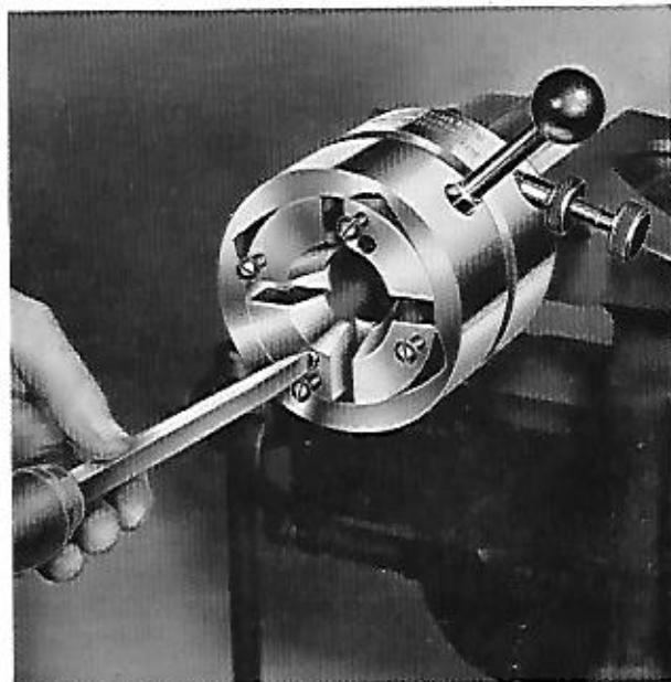
11. Replace the two closing spring screws and springs. Now close the diehead.
