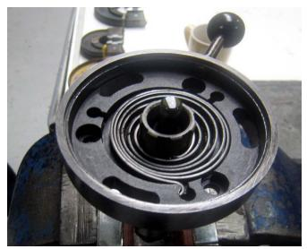
Check that the main coil spring is not broken and that there are no cracks in the spring housing.
