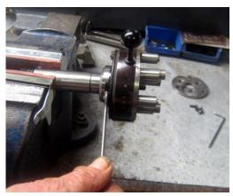
Remove the nuts/washers and ring plate, if fitted, from the spring housing.
