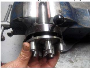
Withdraw the front of the head from the spring housing.
