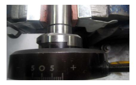
Inspect the 'steps' between the shank and spring housing that lock the diehead closed. If these are worn and rounded the end of the rolled thread will have a taper.
