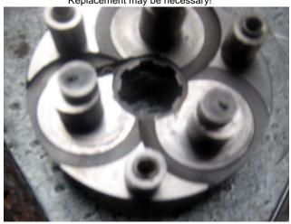
Inspect the eccentric pins for wear or damage.
