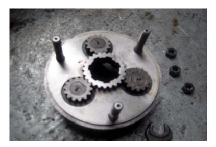
Inspect all parts for wear or damage. Frequent problems include; threads on pillars stripped, teeth missing on gears, gears cracked. The pillars are simply pressed into the back plate so can be knocked out. The outer gears are pressed onto the eccentric pins, they can be removed by tapping the eccentric pin out with a brass drift. The centre gear is held by a circlip. The main coil spring (see below) must be removed to access the circlip.
