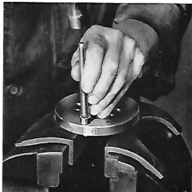
5. With cheese-head screw uppermost, drive the detent pin bush into the back plate using brass rod.
