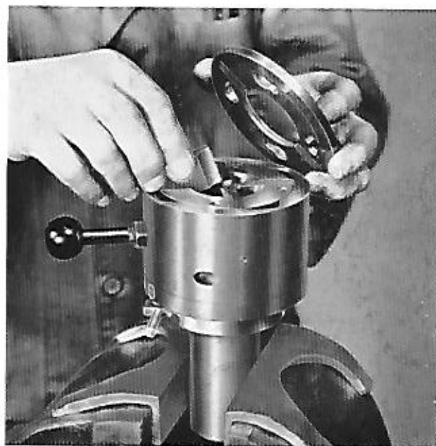
13. Replace the dies and front plate, fixing screws tightly. Put the detent pin handle to the minus position and adjust the diehead to zero.
