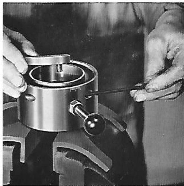
8. Take out the opening spring. Release one of the two adjusting screws and the detent pin tooth can be taken out.
