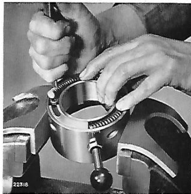
4. Replace the pads in the ends of the opening spring and, using a screwdriver, place the spring in the internal scroll.
