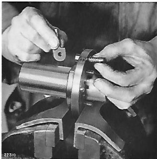
5. Take off the detent-pin nut and handle. Detent pin and spring can now be removed.
