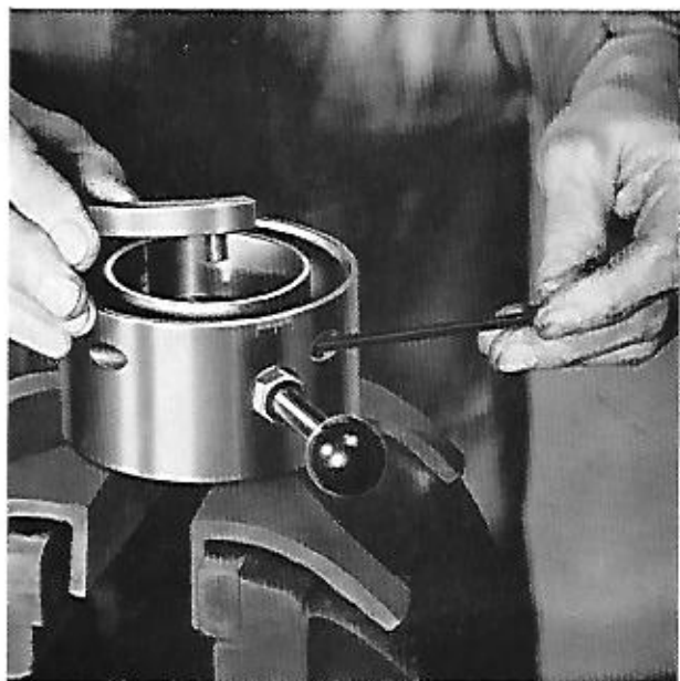
3. Replace the detent pin tooth and lock securely by means of the two adjusting screws.
