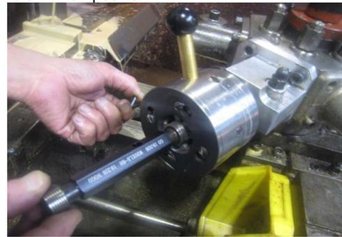
Stops are set on the machine to halt the forward travel of the die head when the thread produced is about 1/8" shorter than that required. When the stop is met the front of the die head will continue to travel forward until the detent pin mechanism is released and the die head will then automatically open.
