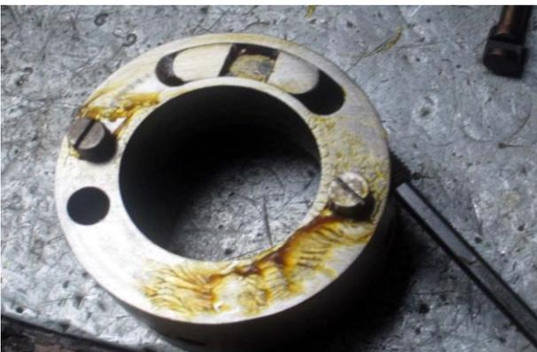
From the external scroll, remove the adjusting screws and tooth.
