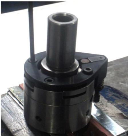
Refit and tighten retaining plate screws.
