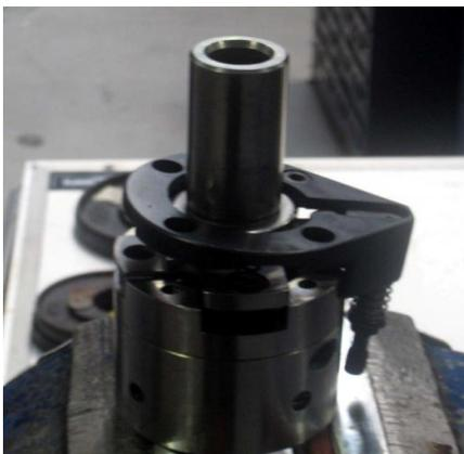
When lifting off retaining plate you should see two outer cushion springs which will become free, note their locations. If instead of springs you find hard rubber pieces these should be replaced by springs. See parts list item 13/14
