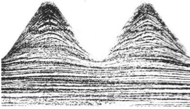
*Thread rolling is essentially a cold forging operation.*
